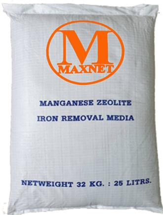
Manganese Zeolite is a granular manganese dioxide filtering media used for reducing iron, manganese and hydrogen sulfide from drinking water. Its active surface coating oxidizes and precipitates soluble iron and manganese. Hydrogen sulfide is oxidized to sulfur. The precipitates are filtered out in the granular bed and removed by backwashing.
